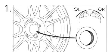
Clean before installation. Tighten the adapter into the center hub bore. The left-hand thread is on the driver's side (LHD).
