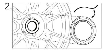
To additionally protect the rim, put rubber on the inside of the plate.
