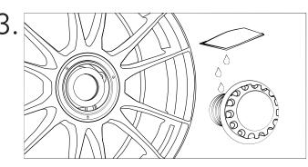
Use a little lubricant on the thread. Tighten the central screw. Use strength 10-15 Nm.
